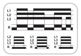
**Phase failure monitoring**When one of the three phases fails, the output relay R switches into off-position (yellow LED not illuminated), after the fixed interval of the tripping delay has expired. Reverse voltages of a consumer (e.g. a motor which continues to run on two phases only) do not effect the disconnection.
